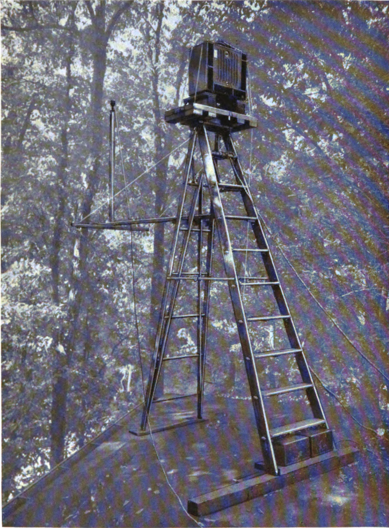
FIGURE 21.— Experimental arrangement for outdoor testing of loudspeakers.
