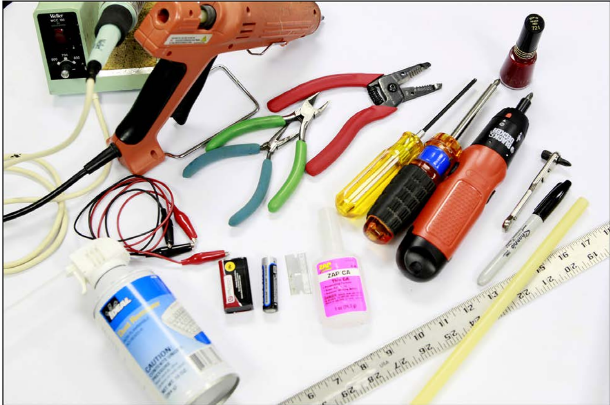
Fig. 3. Tools and consumables required in the assembly of the CBT36. See the following two lists for individual items.
