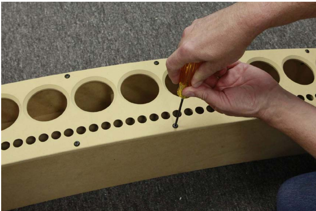
Fig. 4. CBT36 cabinet showing front panel being unscrewed.
