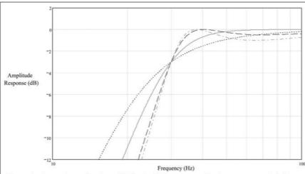
Figure 2: Comparison of various third-order high-pass amplitude responses. -3.0~dB at 30 Hz. — Butterworth; ——— Chebyshev with 0.5-dB ripple;  $-\bullet-$  Chebyshev with 1.0 dB ripple;  $\bullet\bullet\bullet$  Bessel.
