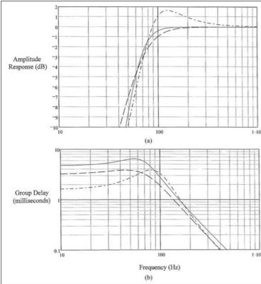
Figure 4: Responses of driver of Table 1, resonance  $F_S = 40$  Hz;  $Q_T = 0.40$ ;  $V_{AS} = 50$  liters. (a) Amplitude versus frequency. (b) Group delay versus frequency. —in 11.2-liter box and with a 900- $\mu$ F capacitor in series, third-order Butterworth response;  $-\bullet-$  in 11.2-liter box without series capacitor; produces second-order response with 1.6-dB peak; ——— in 23.5-liter box without series capacitor, for second-order Butterworth response.
