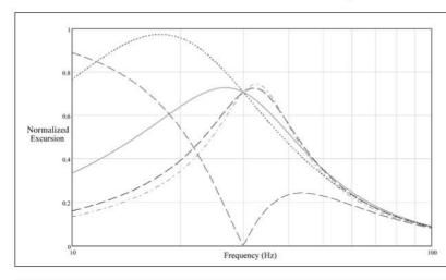
Figure 3: Comparison of driver excursions, various third-order high-pass responses. -3.0 dB at 30 Hz. — Butterworth; ———Chebyshev with 0.5-dB ripple; -•— Chebyshev with 1.0-dB ripple; ••• Bessel; ——— fourth-order high-pass Butterworth, from vented box (for comparison).
