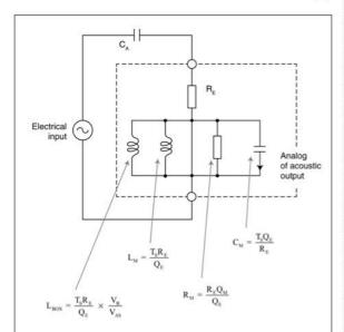
Figure 1: Schematic diagram of a closed-back loudspeaker fed through series capacitance  $C_A$ . Dashed box encloses a model of the driver plus box.  $L_M$ ,  $R_M$ , and  $C_M$ —components of the driver motional impedance;  $L_{BOX}$ —electrical impedance contributed by  $V_B$  box volume.
