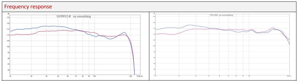
Red line: without horn, blue line: with horn. No smoothing, REW settings: left window 125ms, right window 100ms. Superposition of the curves for the same 114dB level at about 7 kHz.
